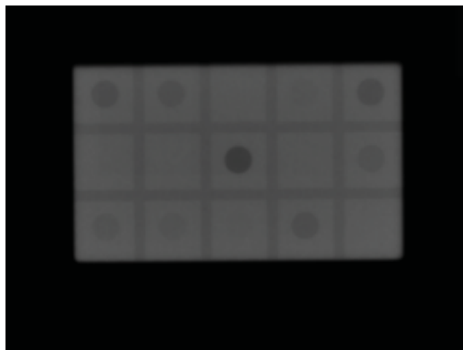
Figure. Radiograph of machined aluminum block developed for perceptibility test.
